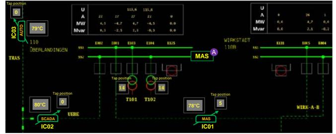
Figure 3: Process visualization of MAS and DPFCs embedded in an exemplary 110 kV grid in PSIcontrol
