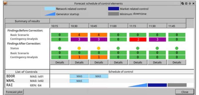
Figure 4: Exemplary Snapshot of Control Actions under Consideration of DPFCs and MAS in PSIcontrol
