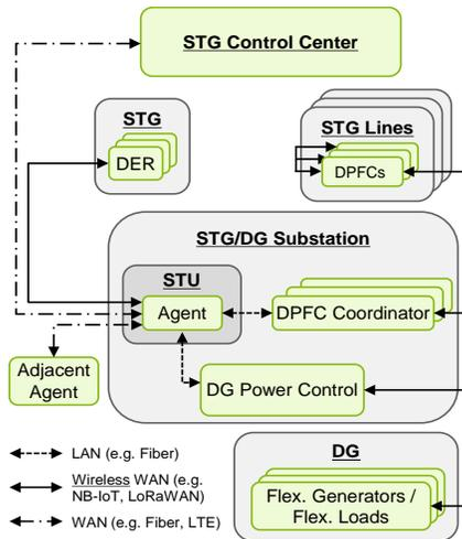
Figure 1: Overview of communication links between system components
